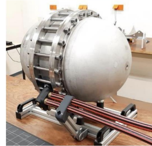
Thermoacoustic heat pump, BHE
